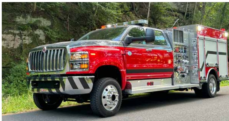
Darley's Tactical Pumper™ shown above equipped with a PSMC 1500 GPM pump, 400 gallon water tank, 25 gallon foam cell, and 120 CFM compressor provides industry leading firefighting capabilities in a compact footprint.
