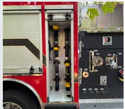
SCBA compartment – 4 bottle holders and 2 pack holders
