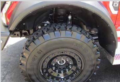
Aluminum rim with aggressive tires to optimize off road drive ability.
