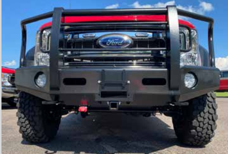
Custom front bumper with driving lights, brushguard & 2" receiver with power portable winch.
