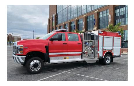
Darley's new Tactical Pumper™ is engineered to safely get to the fire quickly and into places that a full size pumper just can't access. With four wheel drive and a height of approximately 8' tall, this vehicle can get you into those difficult to access driveways. Once on scene, Darley's easy-to-operate AutoCAFS<sup>\*</sup> compressed air foam system packs a punch. Please contact Darley for a full set of specifications or to schedule a demonstration.
