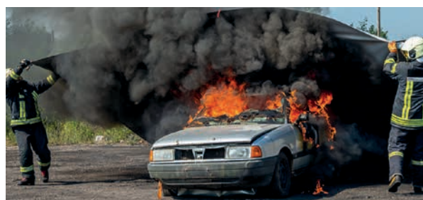
Quickly deploy the car fire blanket with two-people, isolating and containing the spread of fire and toxic smoke.
