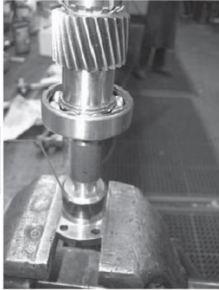
PROPER FIXTURE TO HOLD SHAFT
