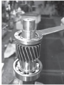
TAB IN SLOT ON LOCK NUT
