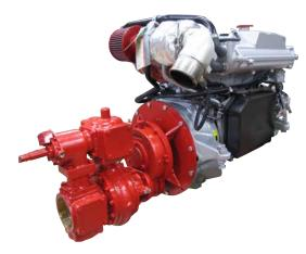
Darley offers bronze pumps with 316 stainless shaft for marine applications. These marine firefighting pumps can be purchased to be fitted to a customer supplied marine engine or can be purchased pre-coupled and tested with a Darley supplied Steyr marine engine.
