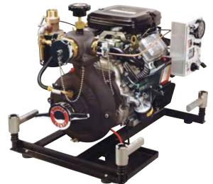
Briggs & Stratton Vanguard: 4 cycle, 23 HP, V-twin, OHV, replaceable oil filter, 12-volt starter, recoil rope start back-up, 16 amp regulated alternator, 6 gal. fuel tank, control panel
