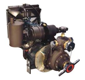
Kubota V1505 Diesel: 42 HP turbo diesel, 4 cylinders, liquid-cooled, 12-volt, electric start, 40 amp alternator, pressure lubed, oil and fuel pump filters
