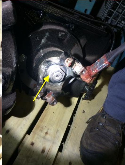
All 7/8-14 interference thread yoke nuts are tightened to 125 ft-lb.
