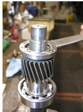
TAB IN SLOT ON LOCK NUT
