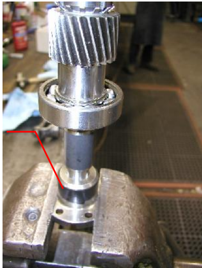
PROPER FIXTURE TO HOLD SHAFT
