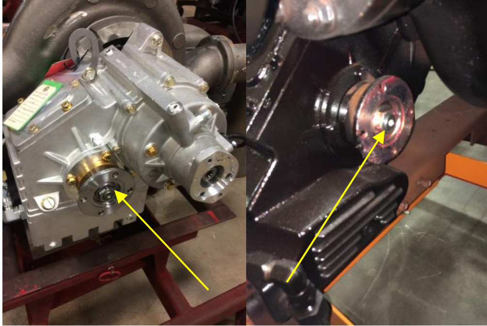
PUC and PUC-3G yoke nuts are tightened to 300-350 lb-ft.
