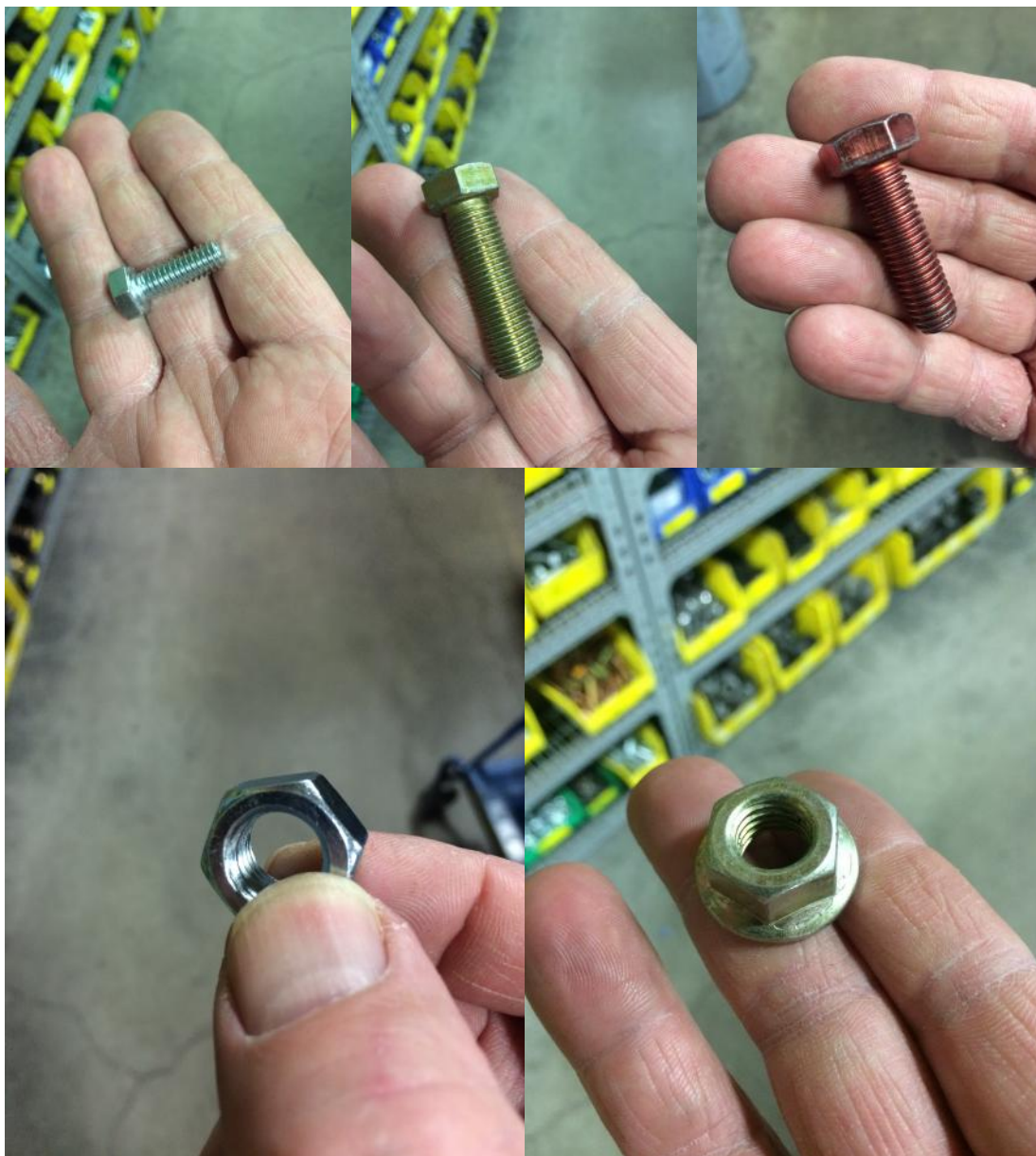
The above images show different types of zinc electroplated fasteners.
