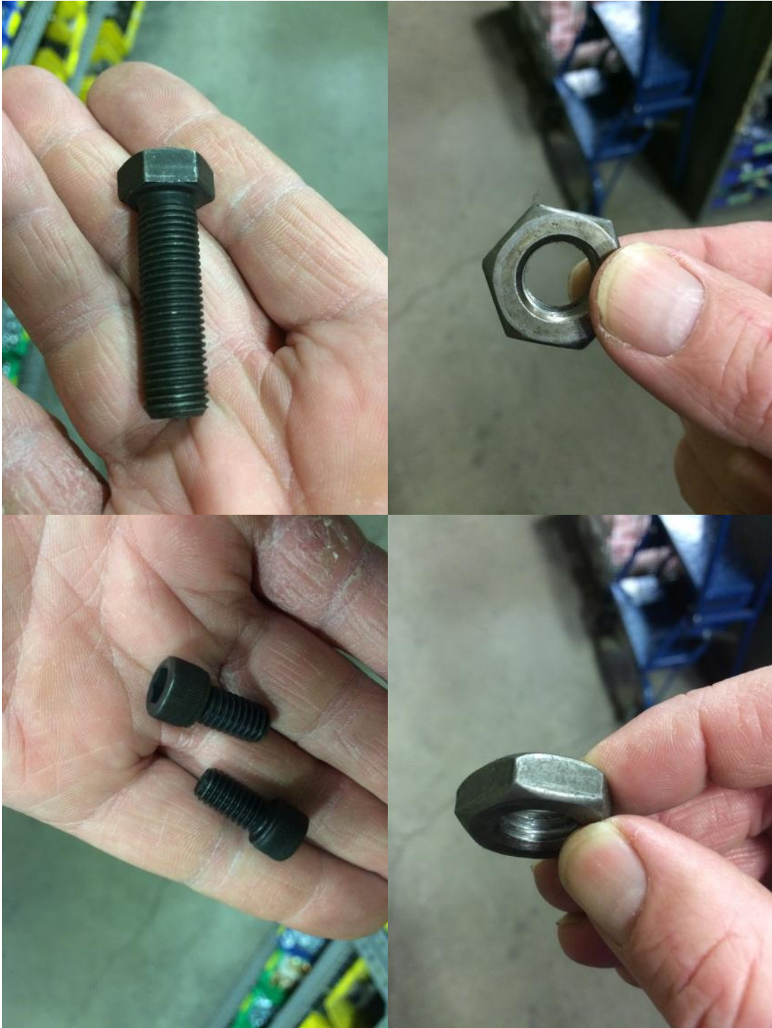
The above images show different types of clean non-plated fasteners.
