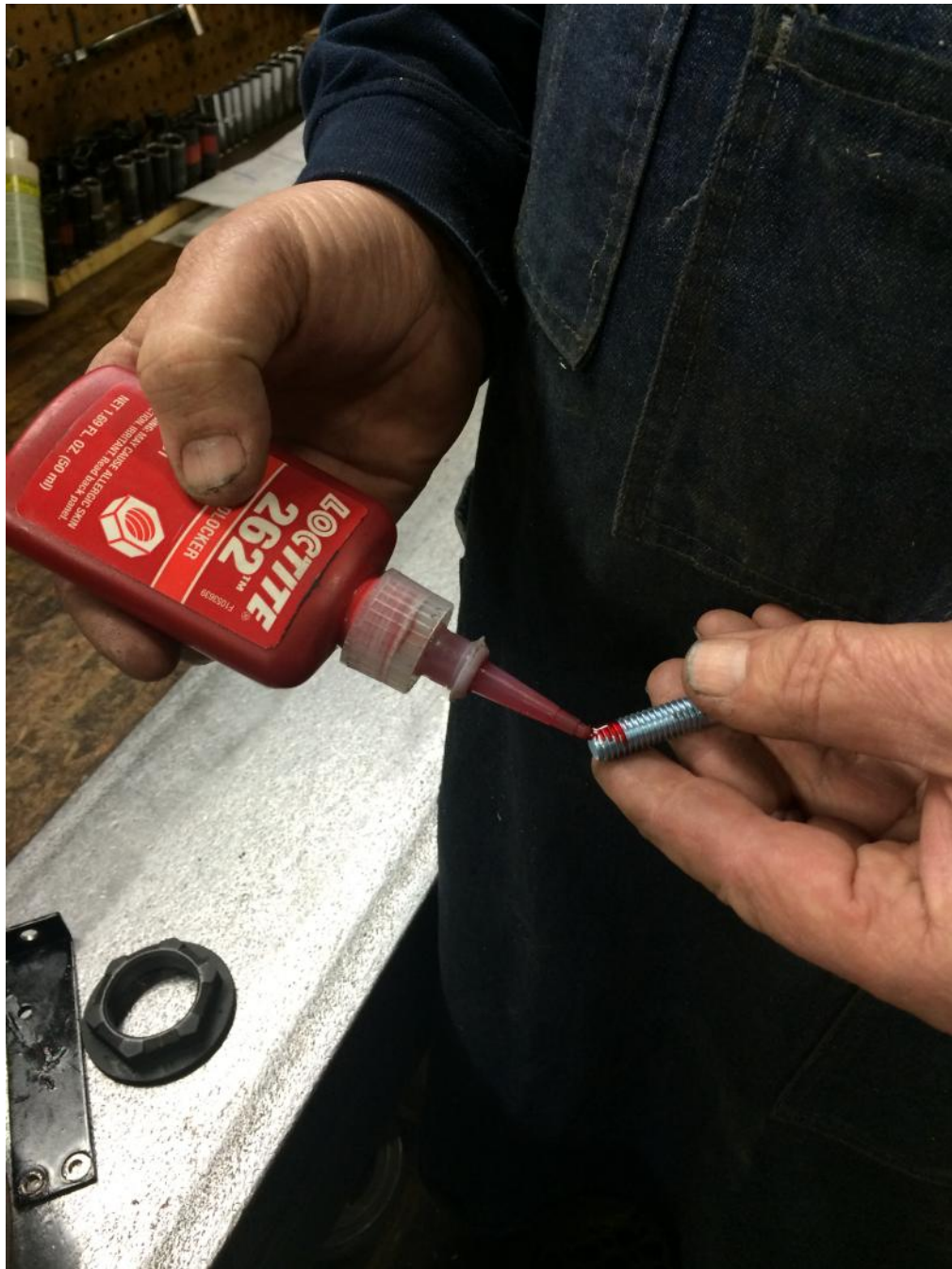
Figure 3 – Apply red Loctite (262) as shown above before installing the fastener.
