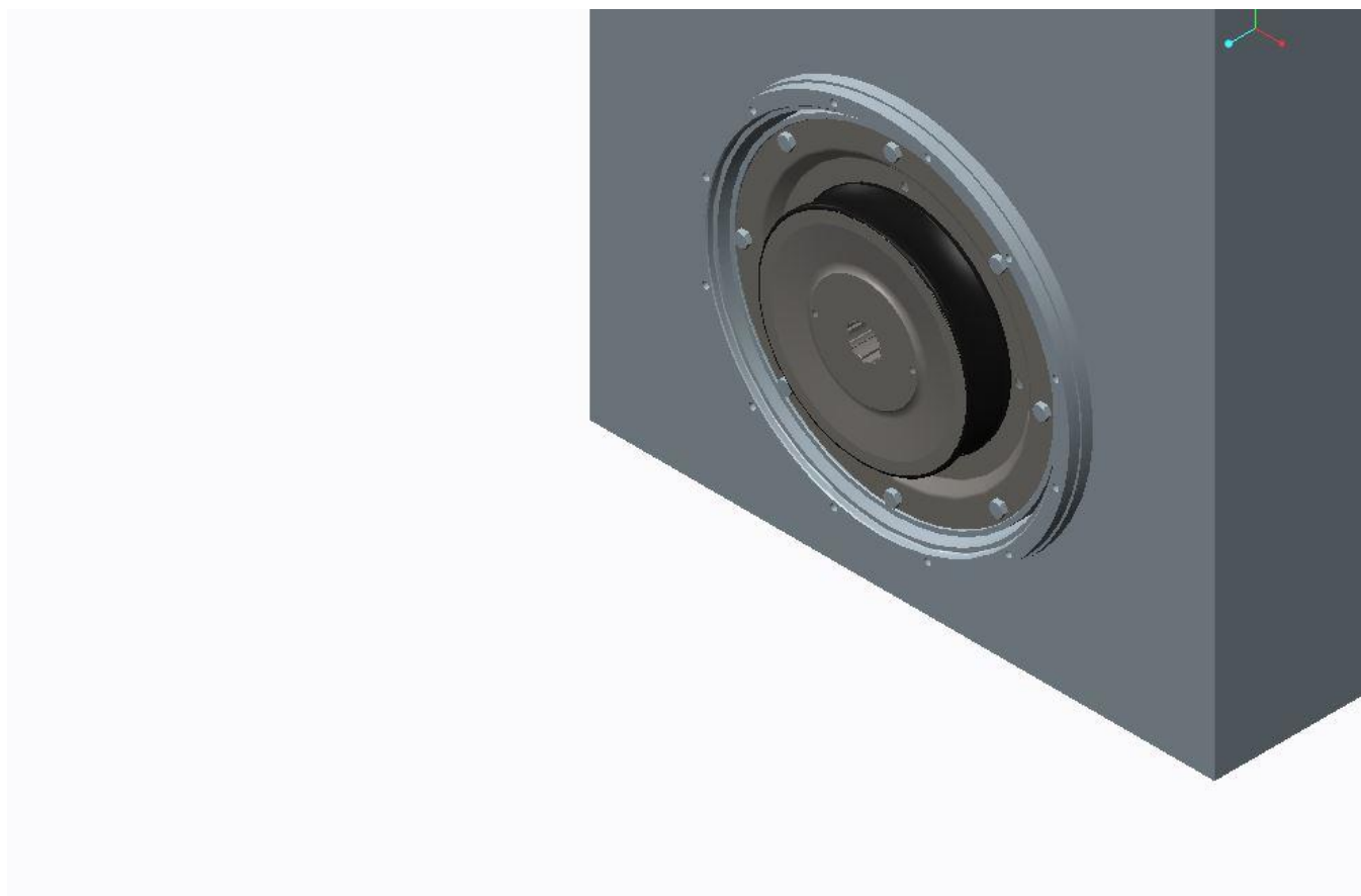
Figure 5 – How the drive disc should look after it has been installed upon the engine's SAE flywheel.
