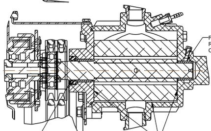
FILL LIP SEAL WITH MULTI-PURPOSE BEARING GREASE PRIOR TO ASSEMBLY
