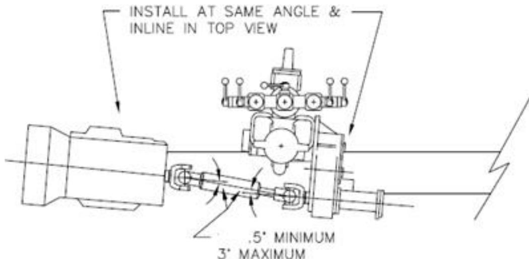
Place suction manifold mounting brackets into position as shown on detail drawing DGM2902 (see next page) and securely clamp against side of frames. Attach brackets to the suction extensions with pipe U-bolts.
