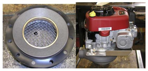
• Remove the rope from the spark plug bore and pull the recoil rope two or three times to align the pump assembly and engine (see photo below).
