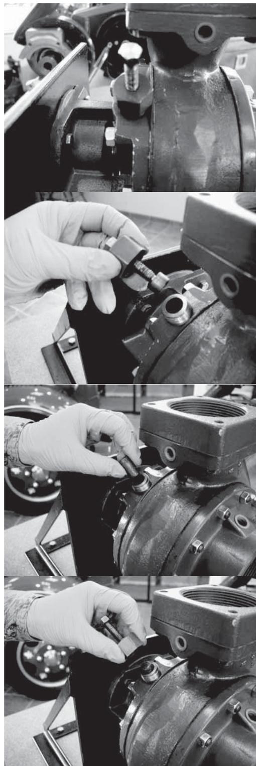
Operate the pump for 10 minutes at the highest normal operating pressure flowing sufficient water to prevent overheating. Do not run the pump blocked tight. Lower discharge pressure to 50 psi and repeat the packing screw tightening procedure outlined above.
