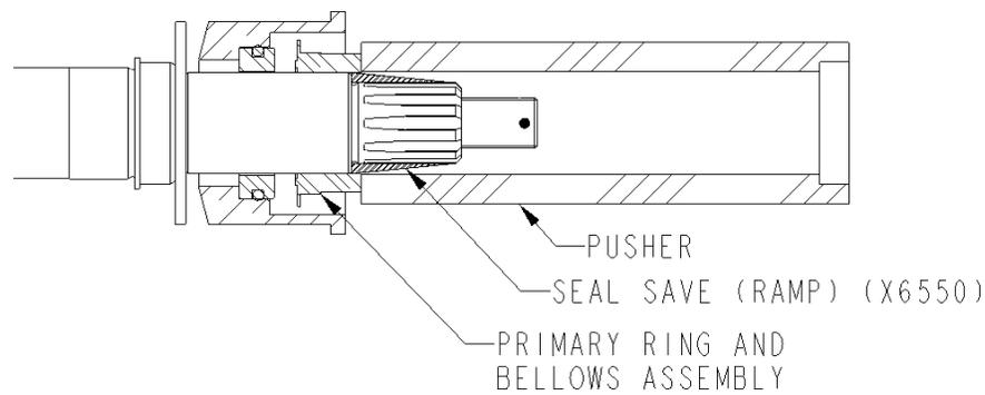
8. Put the spring in place, seated tight against the spring retainer on the primary ring.
