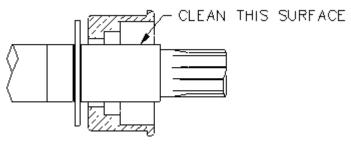
3. Lightly lubricate the entire o-ring on the mating ring with a single drop of P-80 water soluble rubber lubricant evenly distributed (do not over lubricate) and push it into the cavity using the recommended installation tool or other suitable plastic tube free of contaminants, firmly seating the mating ring square. Be careful not to get the P80 on either face. If P-80 is on either face, remove it from the faces prior to installation.
