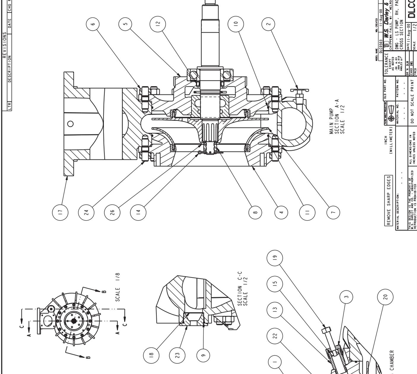
MAIN PUMP SECTION A-A SCALE 1/2
