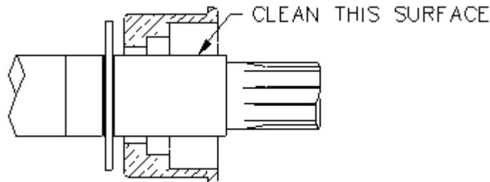
3. Lightly lubricate the entire o-ring on the mating ring with a single drop of P-80 water soluble rubber lubricant - evenly distributed (do not over lubricate) and push it into the cavity using the recommended installation tool or other suitable plastic tube free of contaminants, firmly seating the mating ring square. Be careful not to get the P80 on either face. If P-80 is on either face, remove it from the faces prior to installation.
