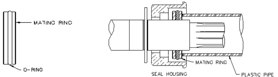
4. Clean the mating ring surface with isopropyl alcohol to remove any fingerprints and any other contaminants left on mating ring.
