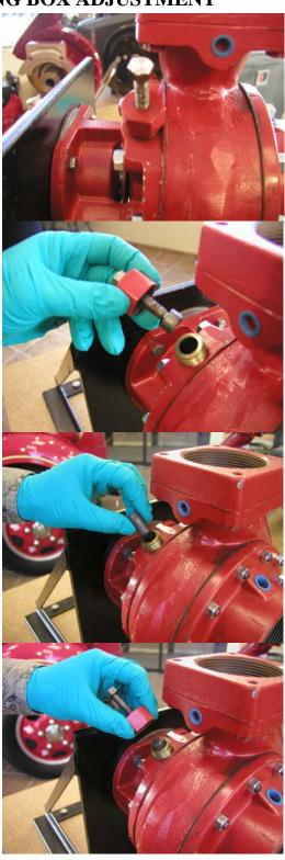
Prepared by: TED Approved by: MCR Revised by: AAN Rev. #: 3 Date: 10June2003 1200504 Operate the pump for 10 minutes at the highest normal operating pressure flowing sufficient water to prevent overheating. Do not run the pump blocked tight. Lower discharge pressure to 50 psi and repeat the packing screw tightening procedure outlined above.
