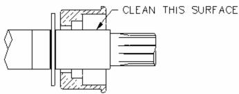
3. Lightly lubricate the o-ring on the mating ring with a single drop of P-80 water soluble rubber lubricant (do not over lubricate) and push it into the cavity using the recommended installation tool or other suitable plastic tube free of contaminants, firmly seating the mating ring square.
