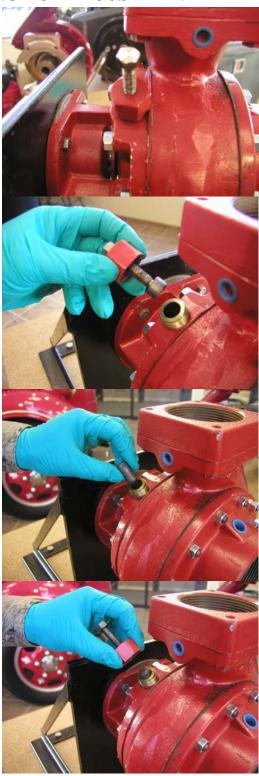
Prepared by: TED Approved by: MCR Revised by: AAN Operate the pump for 10 minutes at the highest normal operating pressure flowing sufficient water to prevent overheating. Do not run the pump blocked tight. Lower discharge pressure to 50 psi and repeat the packing screw tightening procedure outlined above.
