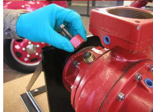
Operate the pump for 10 minutes at the highest normal operating pressure flowing sufficient water to prevent overheating. Do not run the pump blocked tight. Lower discharge pressure to 50 psi and repeat the packing screw tightening procedure outlined above.
