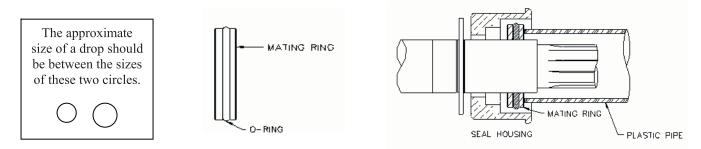
4. Clean the mating ring surface with isopropyl alcohol to remove any fingerprints and any other contaminants left on mating ring.
