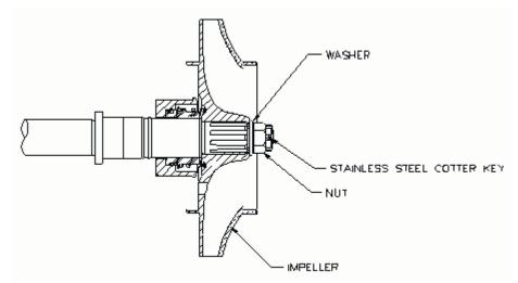
\*\* Reference pump configuration for individual mechanical seal instructions. \*\* Reference pump assembly drawings and pump assembly tips for further assembly.
