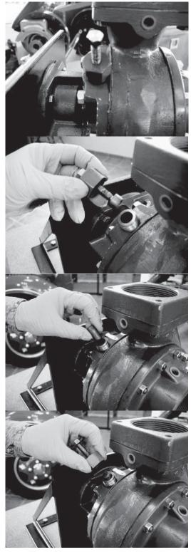
Rev. 22 Date: 06/27/05 Rev Date: 07/28/10 1200536.doc Operate the pump for 10 minutes at the highest normal operating pressure flowing sufficient water to prevent overheating. Do not run the pump blocked tight. Lower discharge pressure to 50 psi and repeat the packing screw tightening procedure outlined above.
