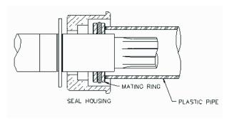
4. Clean the mating ring surface with isopropyl alcohol to remove any fingerprints and any other contaminants left on mating ring.
