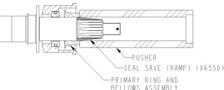
8. Put the spring in place, seated tight against the spring retainer on the primary ring. Note: Some springs may be slightly tapered, so one end fits the seal better than the other. The end of the
