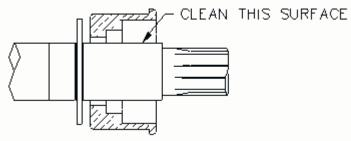
3. Lightly lubricate the o-ring on the mating ring with a single drop of P-80 water soluble rubber lubricant (do not over lubricate) and push it into the cavity using the recommended installation tool or other suitable plastic tube free of contaminants, firmly seating the mating ring square.
