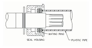
4. Clean the mating ring surface with isopropyl alcohol to remove any fingerprints and any other contaminants left on mating ring.
