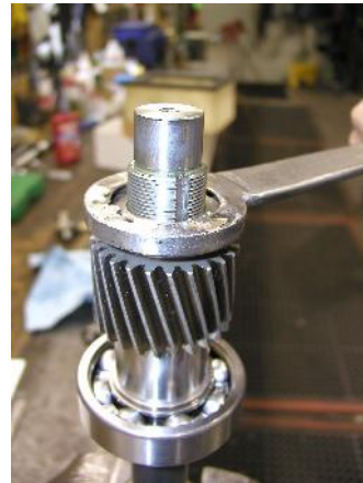
TAB IN SLOT ON LOCK NUT
