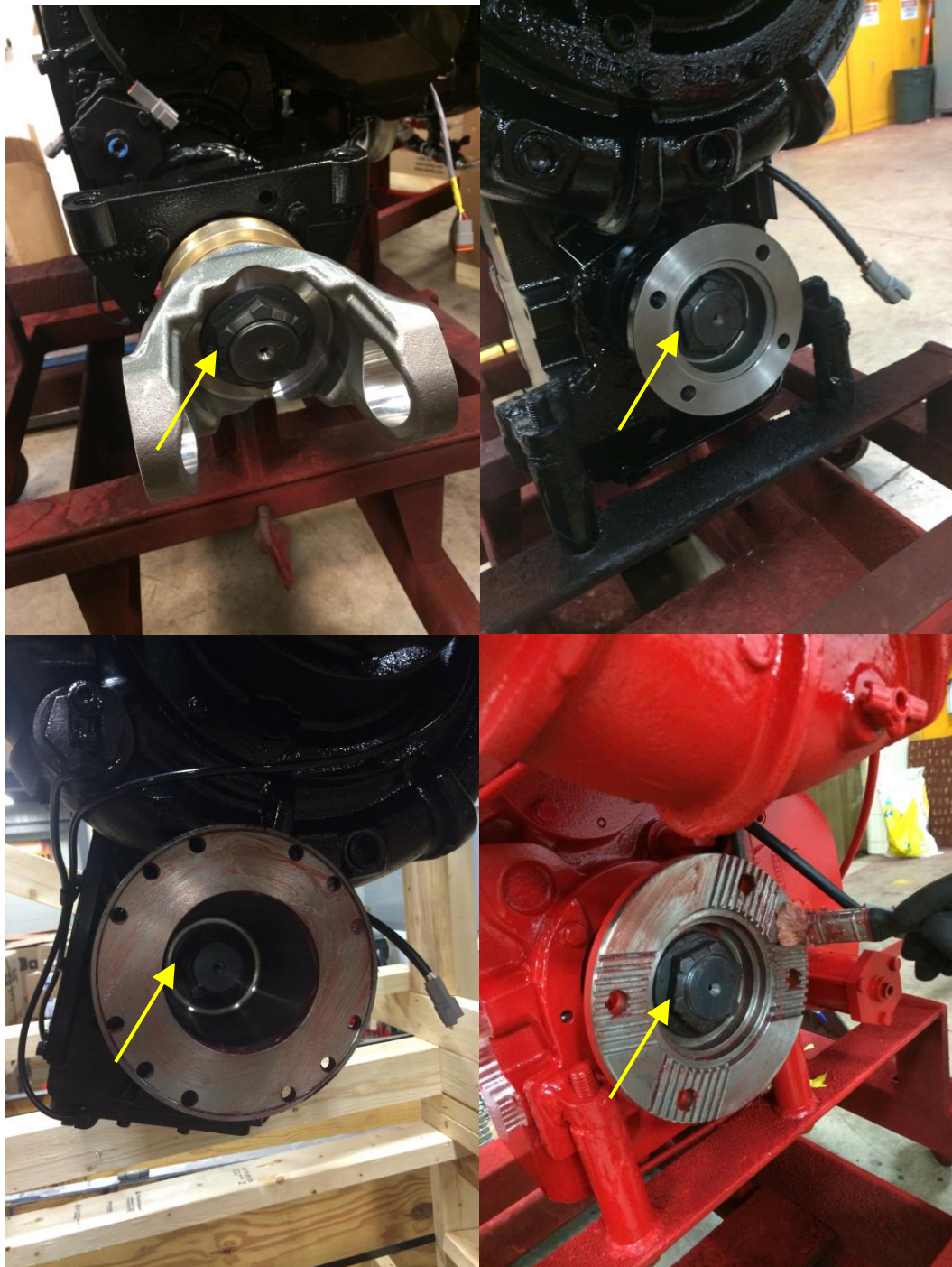
All 1.75-12 interference threaded yoke nuts are torqued to 150-200 ft-lb.
