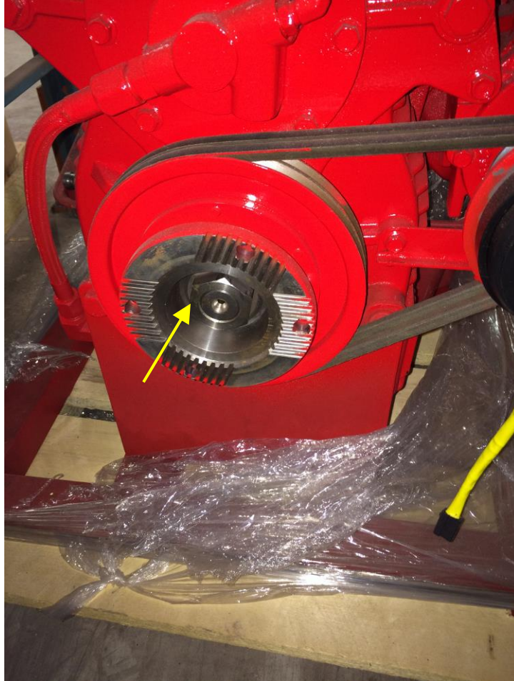
All 1.25-12 threaded yoke nuts are torqued to 150-200 ft-lb.
