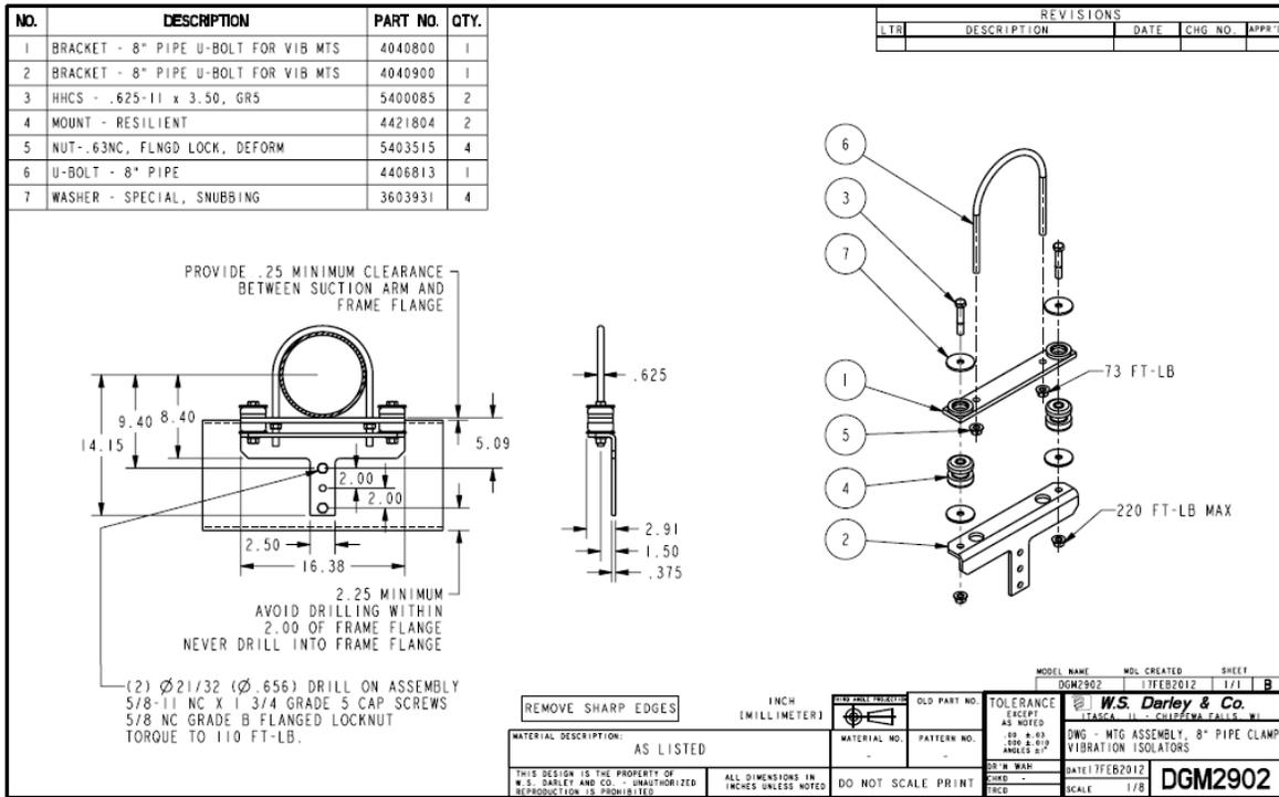
One of the two suction manifold brackets must be free to pivot as seen in drawing DGM1302. Choose one side of the frame or the other for the location of the pivot, the opposite must be rigidly secured with (2) 5/8" fasteners.
