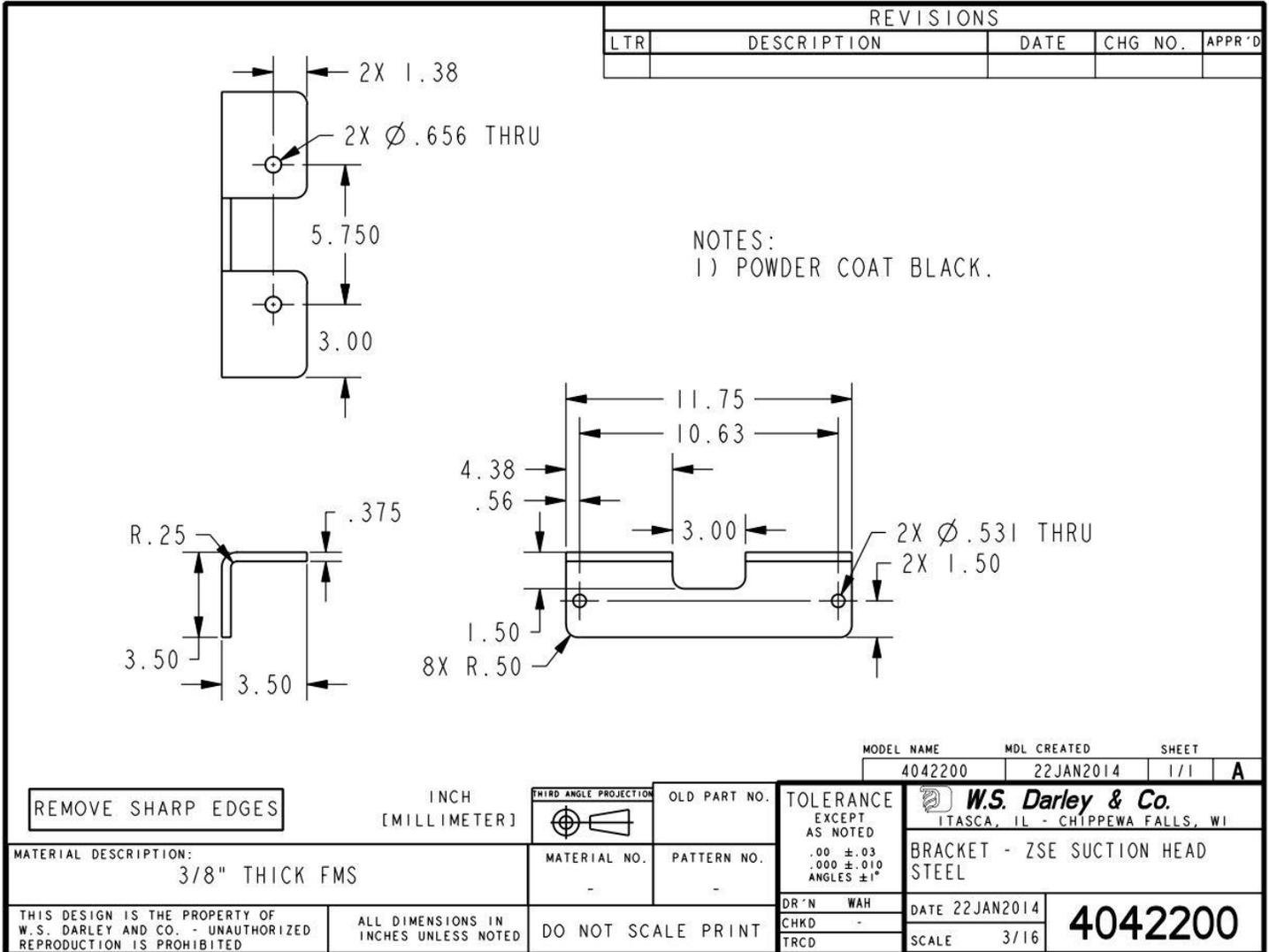
The 4042200 bracket is intended to be secured with 1/2" fasteners or welded back to the customers bracketing and cross members.
