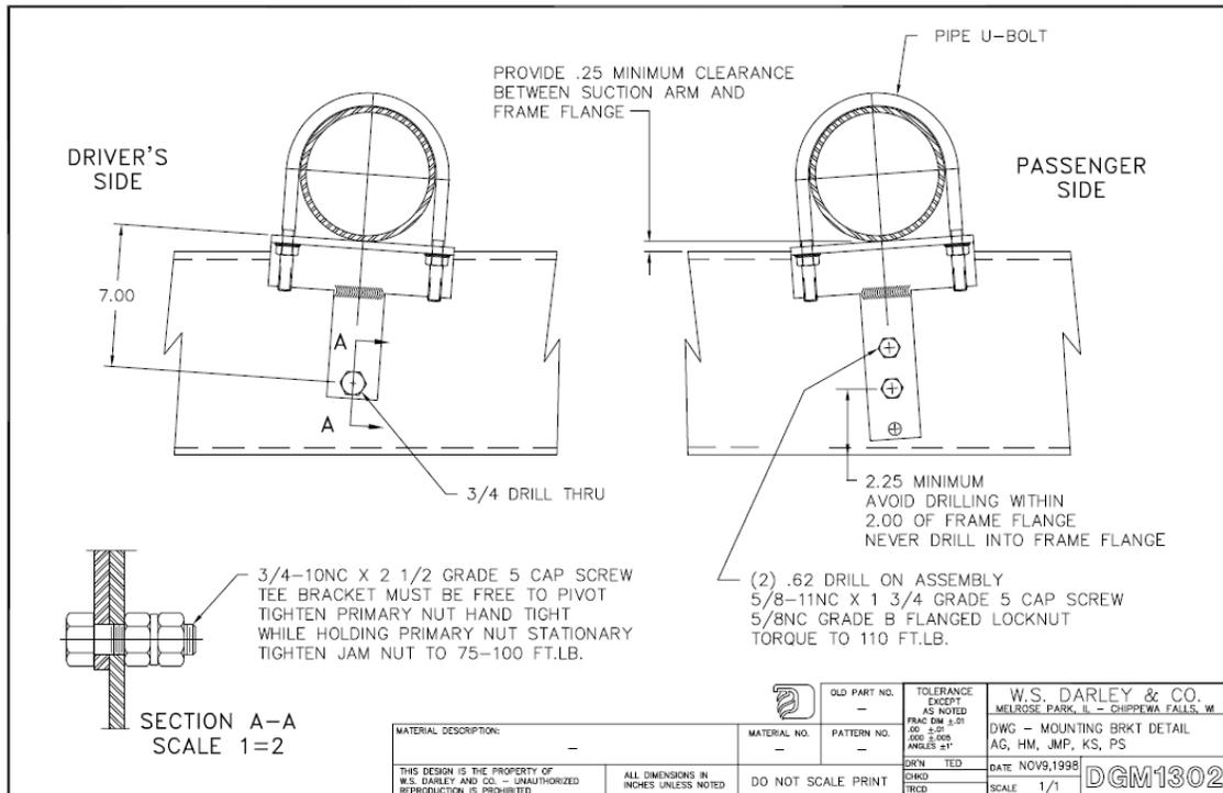
Drill holes through the side frames and attach the mounting brackets. Note both mounting brackets are designed to permit truck frame flex without imposing stress on pump extensions.
