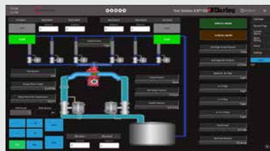
Mounted on movable carts, the new control screen allows test technicians to adjust the RPM, ball valve, and suction valves while working on other duties.
