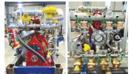
The rear mount PSRH with MegaTrans is capable of flows up to 2000 GPM.
