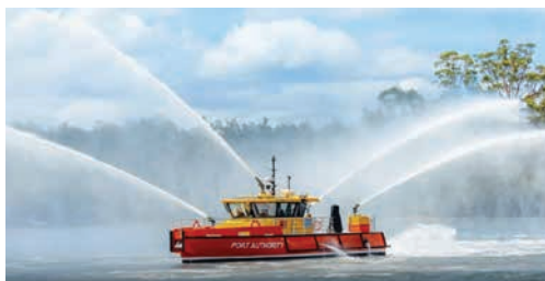
Two new firefighting vessels for New South Wales are equipped with two Darley PSP 2000 pumps, flowing over 5000 GPM.
