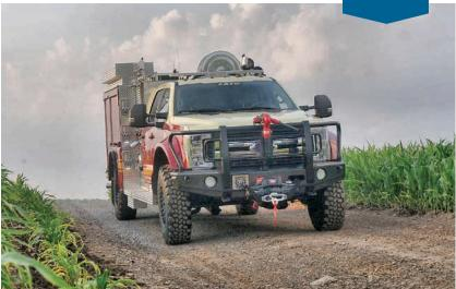
Equipped with Darley's Super Single Tire & Wheel Package, the new Max Tactical Pumper™ is engineered to safely get to the fire quickly and into places that a full-size pumper just can't access. Upgraded taller tires on DOT rated wheels get the most power to the ground through all speed ranges and the lift package increases ground clearance for better off-road capability.
