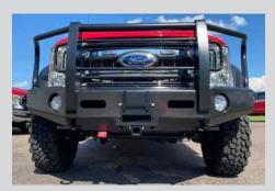
Custom front bumper with driving lights, brushguard & 2" receiver with power portable winch.
