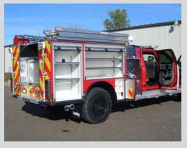
A spacious hosebed and large rear compartment finish off the back of this pumper.
