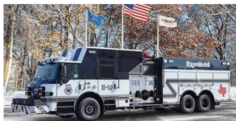
An industrial setting requires fire trucks to flow a high volume of pressured water and foam at an extremely high rate of speed to elevated storage tanks and large processing facilities.
