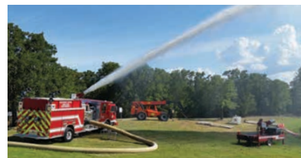
The Darley 2ZSM (shown here during testing) pumped for days helping to contain the fire at the Dow Chemical Plant in Iberville, LA.
