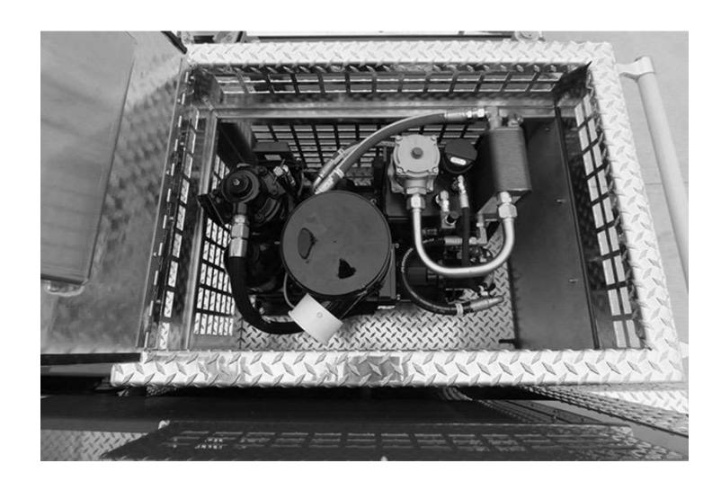
Pierce Manufacturing Inc. located this Hercules CAFS 140-cfm hydraulic system on top of this pumper above the pump house. (*Photo 2 courtesy of Pierce Manufacturing Inc.*)
