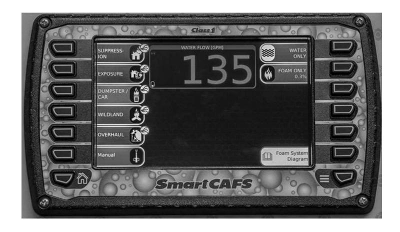
**3** The touch screen control panel for a Hale SmartCAFS unit made by Hale Products, an IDEX Fire & Safety Division. (*Photo 3 courtesy of Hale Products.*)
