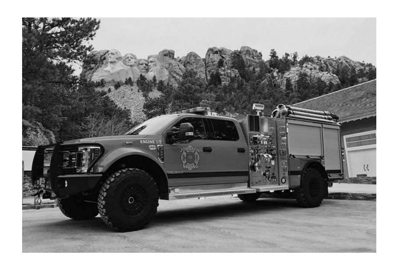
**1** W.S. Darley & Company built this MaxWASP Type 6 pumper for the Johnson Siding (SD) Fire Department with a Darley PSMC 1,500-gpm pump, a 120-cfm rotary screw CAFS air compressor, and a FoamPro 2001 foam proportioner. (*Photo 1 courtesy of W.S. Darley & Company.*)
