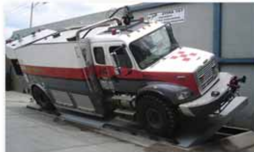
Quiroga has invested in a tilt table for NFPA 1901 testing.
