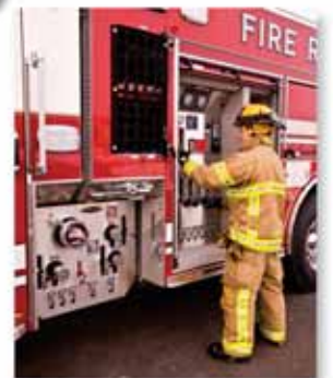
The PUC Pump controls are out of the way of the operator allowing for easy access and safety.
