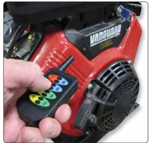
Darley's new smart control allows full pump engine operation from inside the cab or any location up to 75 feet away.
